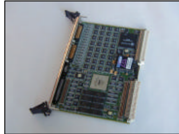
ICS-145 32-ch. 16-bit oversampling ADC board with 2.5 MHz/ch. simultaneous sampling (Download Tech Note #32)
