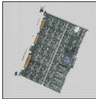
ICS-131 32-ch. signal conditioning and gain board with bandwidth of up to 570 kHz (Download Tech Note #34)
